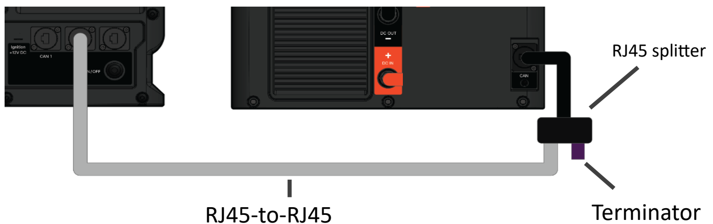
Figure 6 CAN communication between e-Power and e-Heater
