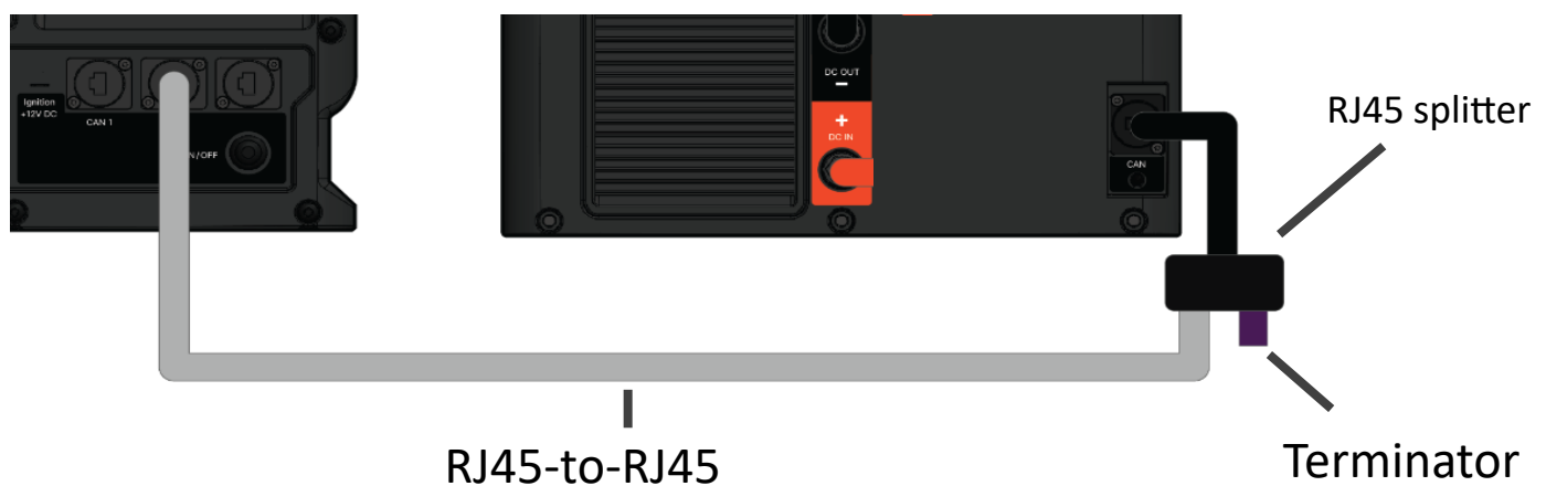
Figure 6 CAN communication between e-Power and e-Heater
